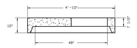
REINFORCING SHALL CONFORM TO A. S. T. M. DESIGNATION C-478 PRECAST, REINFORCED, CONCRETE SECTIONS.
